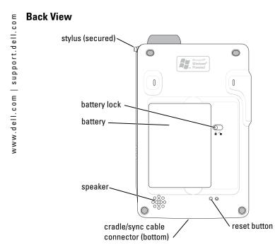
**BATTERY LOCK**—Use this switch to release and remove the main battery. See "Installing and Removing the Battery" on page 21.
